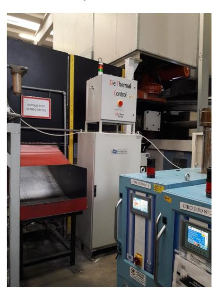
Panel PC positioned to operator side on mobile arm and electropneumatic cabinet installed on wall or on raised support
